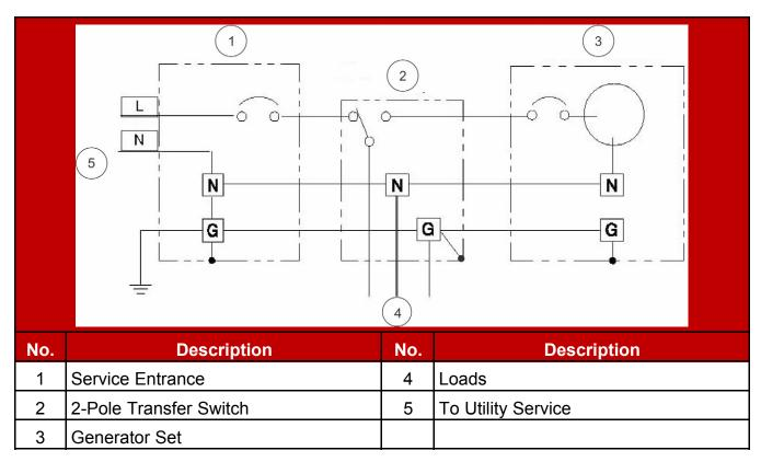
FIGURE 15. TYPICAL SYSTEM GROUNDING ONE-LINE DIAGRAM (SEPARATE SERVICE ENTRANCE AND 2-POLE TRANSFER SWITCH)
