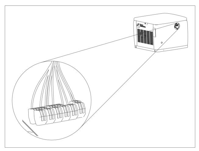
FIGURE 14. LOCATION OF CONNECTION POINTS FOR ATS DC CONTROL WIRES
