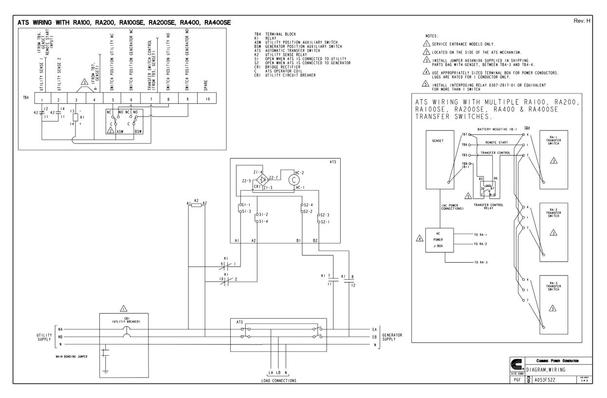
FIGURE 41. WIRING DIAGRAM (SHEET 3 OF 6)
