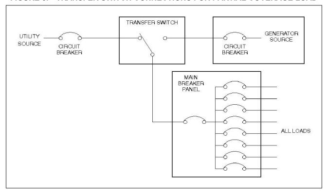
FIGURE 4. TRANSFER SWITCH CONNECTIONS FOR FULL COVERAGE LOAD
