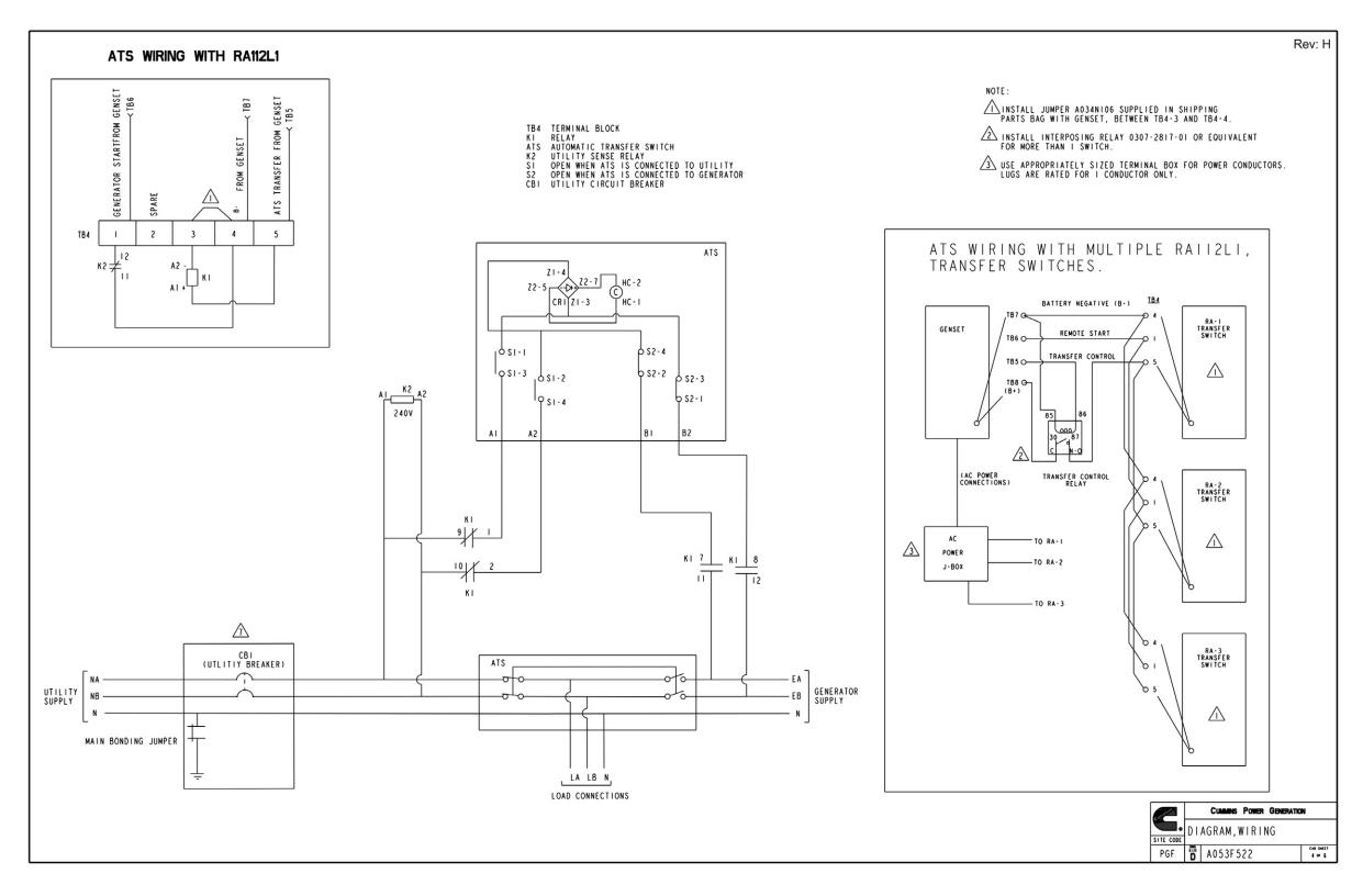
FIGURE 42. WIRING DIAGRAM (SHEET 4 OF 6)
