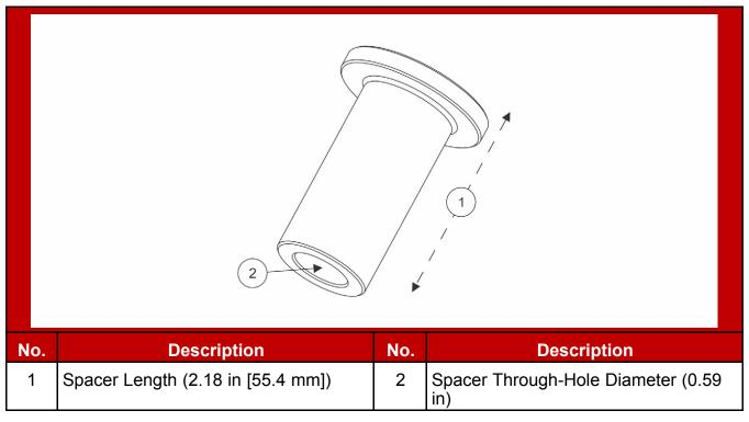
FIGURE 5. MOUNTING SPACER
