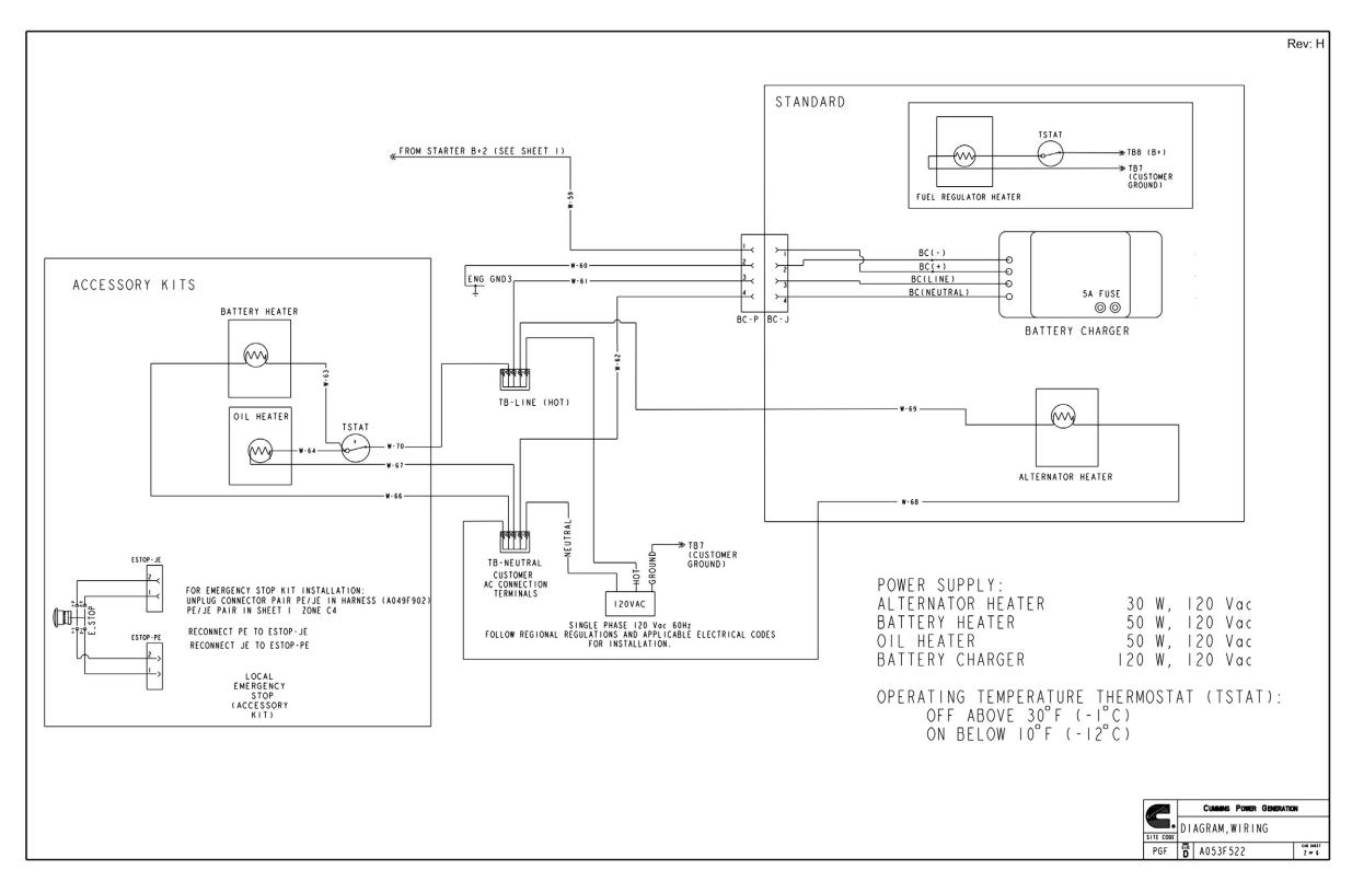
FIGURE 40. WIRING DIAGRAM (SHEET 2 OF 6)
