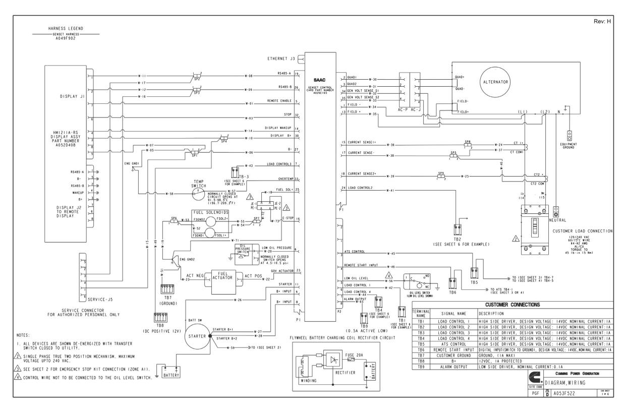
FIGURE 39. WIRING DIAGRAM (SHEET 1 OF 6)
