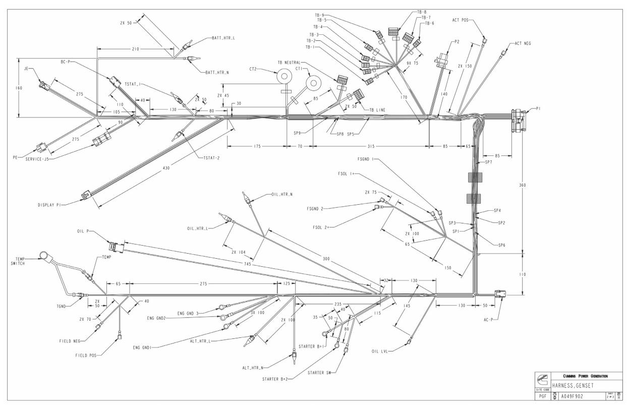
FIGURE 46. HARNESS, GENERATOR SET ELECTRICAL (SHEET 2 OF 3)
