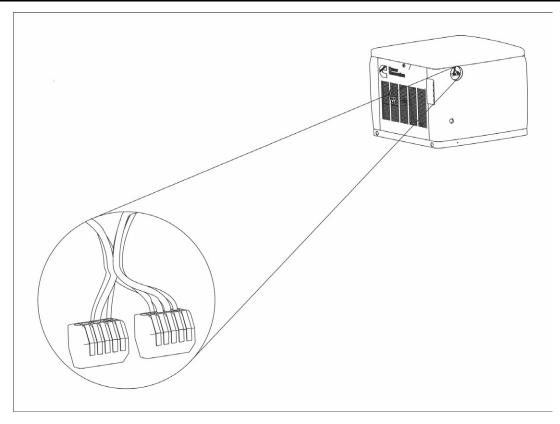
FIGURE 13. CUSTOMER AC CONNECTIONS
