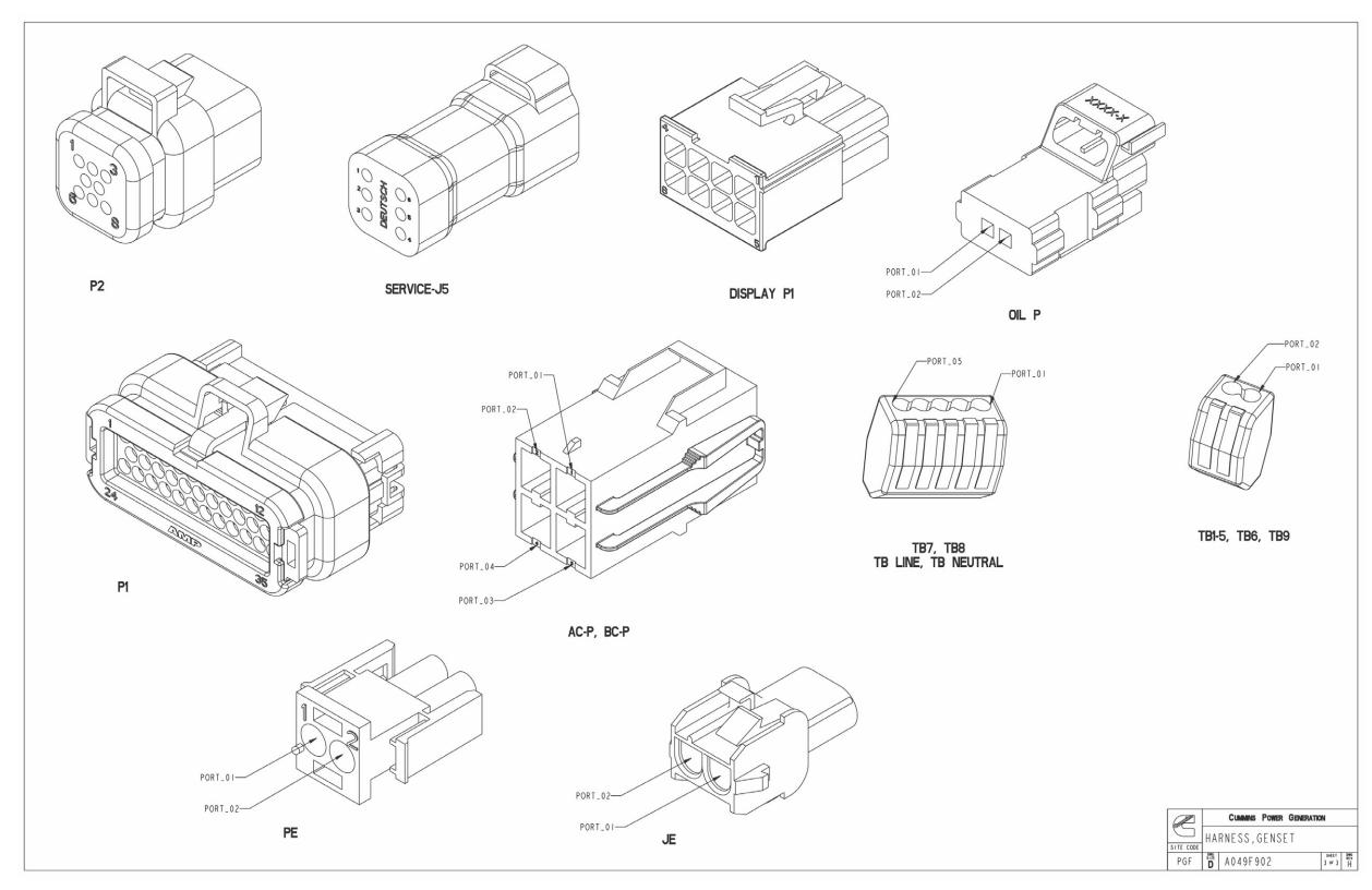
FIGURE 47. HARNESS, GENERATOR SET ELECTRICAL (SHEET 3 OF 3)
