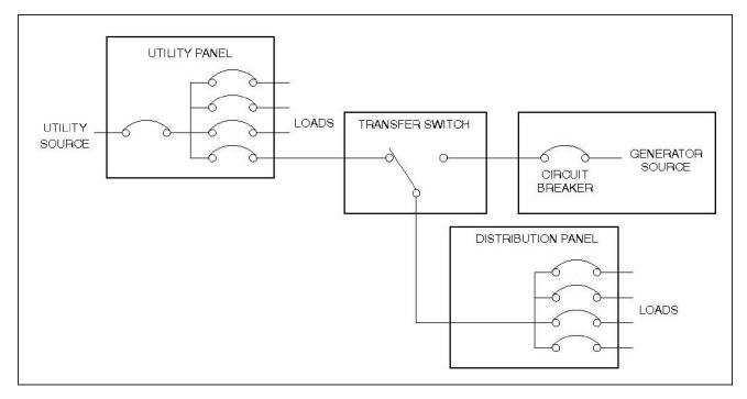
FIGURE 3. TRANSFER SWITCH CONNECTIONS FOR PARTIAL COVERAGE LOAD
